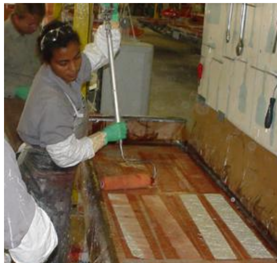
Using a Power Roller for fiberglass wet out.
