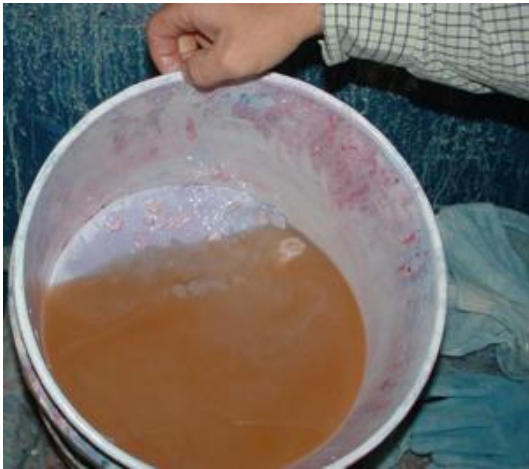
This 5 gallon bucket is 1/2 full of gelcoat sludge. Pour the liquid Bio-Solv off for reuse.
