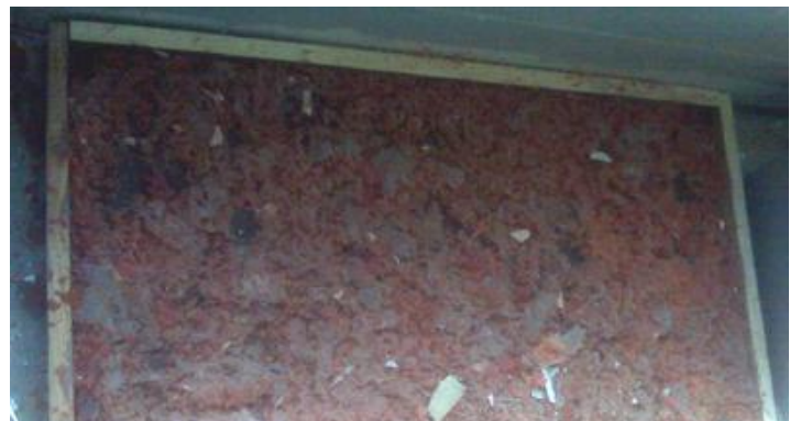
Pans are dumped into a shallow tray and material is spread out to cure to a solid for disposal.
