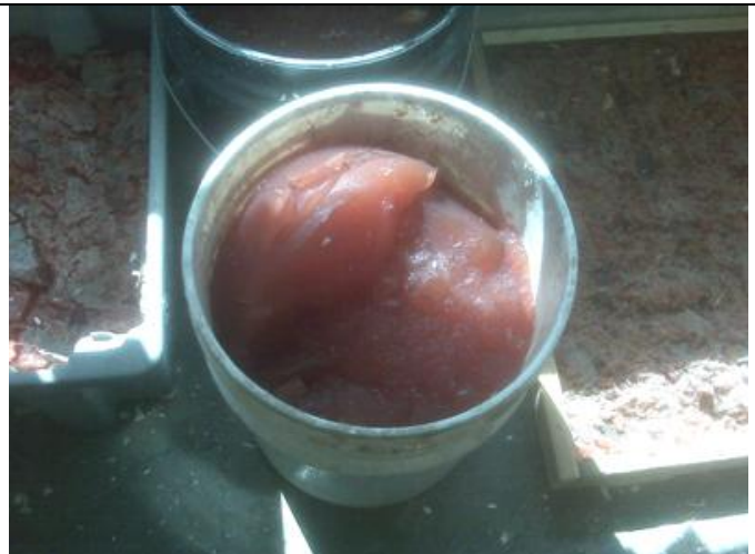
This 5 gallon bucket contains gelled resin sludge from line flushing – about the consistency of stiff Jell-O.
