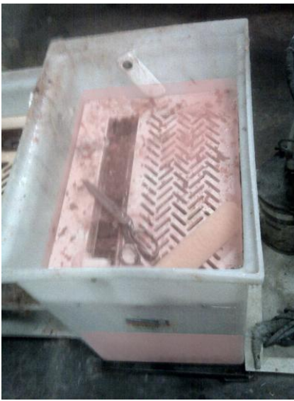
10 gallon cleaning station used to clean tools and allow Sludge to settle to the bottom.
