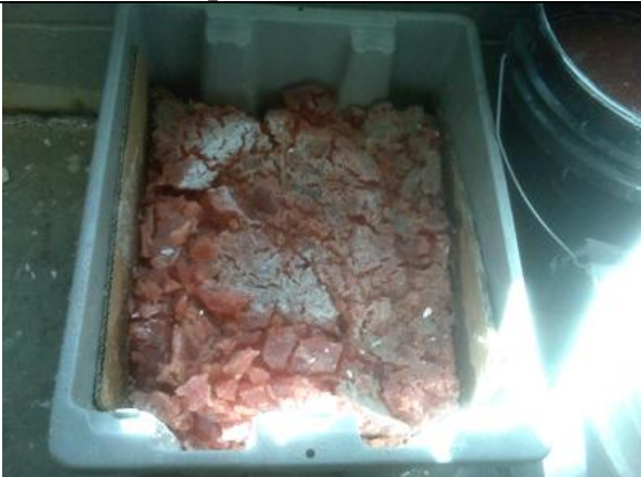
Workers dump the sludge buckets into pans to increase surface area speeding curing time.
